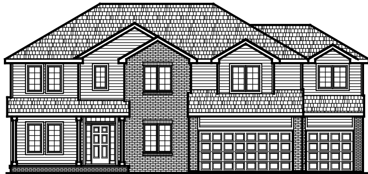
FRONT ELEVATION WITH SUN RM & HIP ROOF (SHOWN WITH OPTIONAL GRILLS BTWN GLASS)
